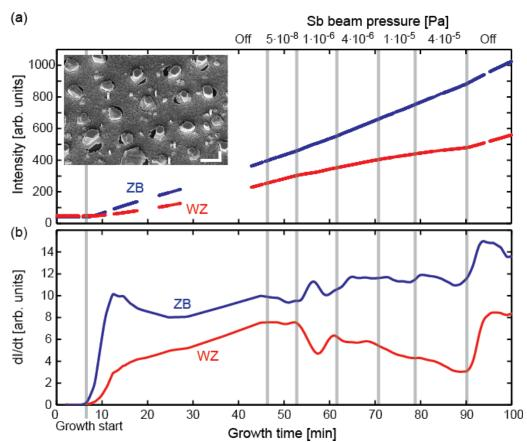
amounts of Sb influences the growth of Au-assisted InAs NW growth<sup>iii</sup>, but the new study for self-assisted NWs shows that also the total growth rate is affected by the introduction of Sb.
