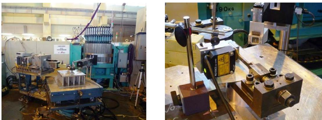
Fig. 2.2 Neutron diffraction experiment at RESA-1 (left) and specimen in tensile jig (right).
