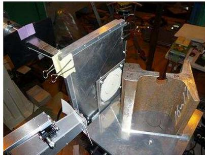
Fig.1 Slit ant its set-up for neutron stress evaluation in rail.
