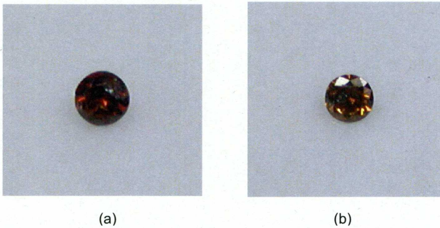
Fig. 2 Photos of reddish diamonds produced by proton irradiation and subsequent annealing at 600°C in vacuum for 2 hours: (a) dark green changes to strong reddish color. (b) white brown diamond shows brighter and rather brownish color.
