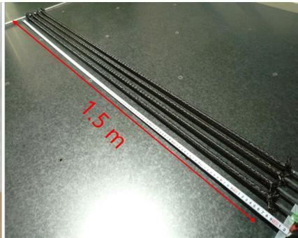
SiC Cladding tube Preform
