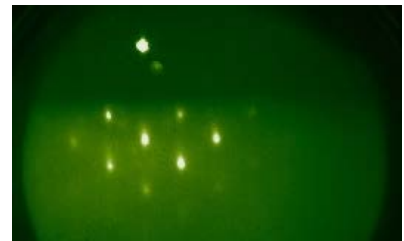
Figure 2 – RHEED pattern showing the growth of crystalline GaAs(001) on MnSb(1-101)
