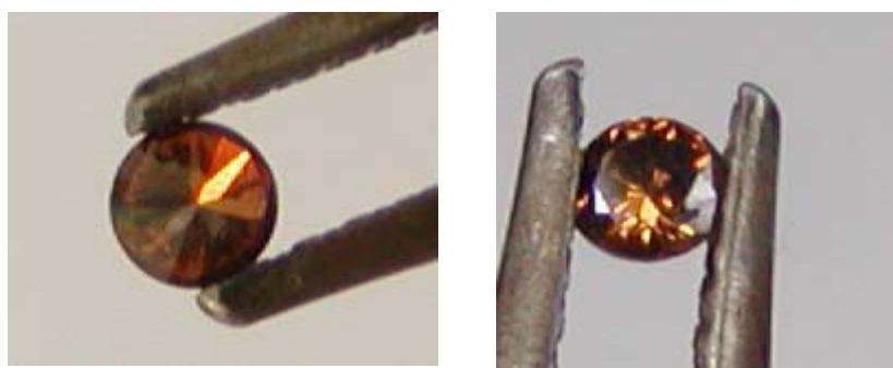
Fig. 2 Photo of a yellow-red diamond produced by proton ( H^+ ion) irradiation and subsequent annealing at 600^{\circ}C in vacuum for 2 hours.
