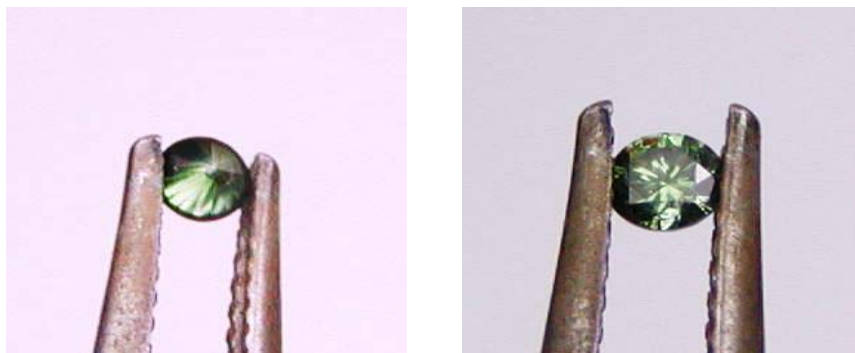
Fig. 1 Photo of a green colored diamond produced by 2 MeV proton ( H^+ ion) implantation.
